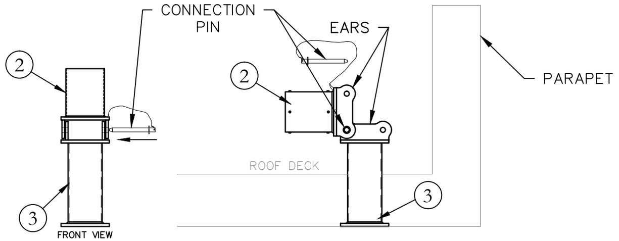
1. MOVE THE SOCKET ASSEMBLY (#2) INTO THE DAVIT BASE (#3) AS SHOWN. ALIGN THE HOLES OF THE SOCKET ASSEMBLY (#2) WITH THE HOLES OF THE DAVIT BASE (#3) AND INSTALL THE 1"Ø CONNECTION PIN SO THAT THE SOCKET ASSEMBLY (#2) CAN BE TIPPED AWAY FROM THE ROOF EDGE. EARS SHOULD SEAT COMPLETELY WITHIN THE OTHER SET OF EARS AS SHOWN IN THE FRONT VIEW. MAKE SURE THE CONNECTION PIN SAFETY CLIP IS INSTALLED AND IS FULLY ENGAGED.
