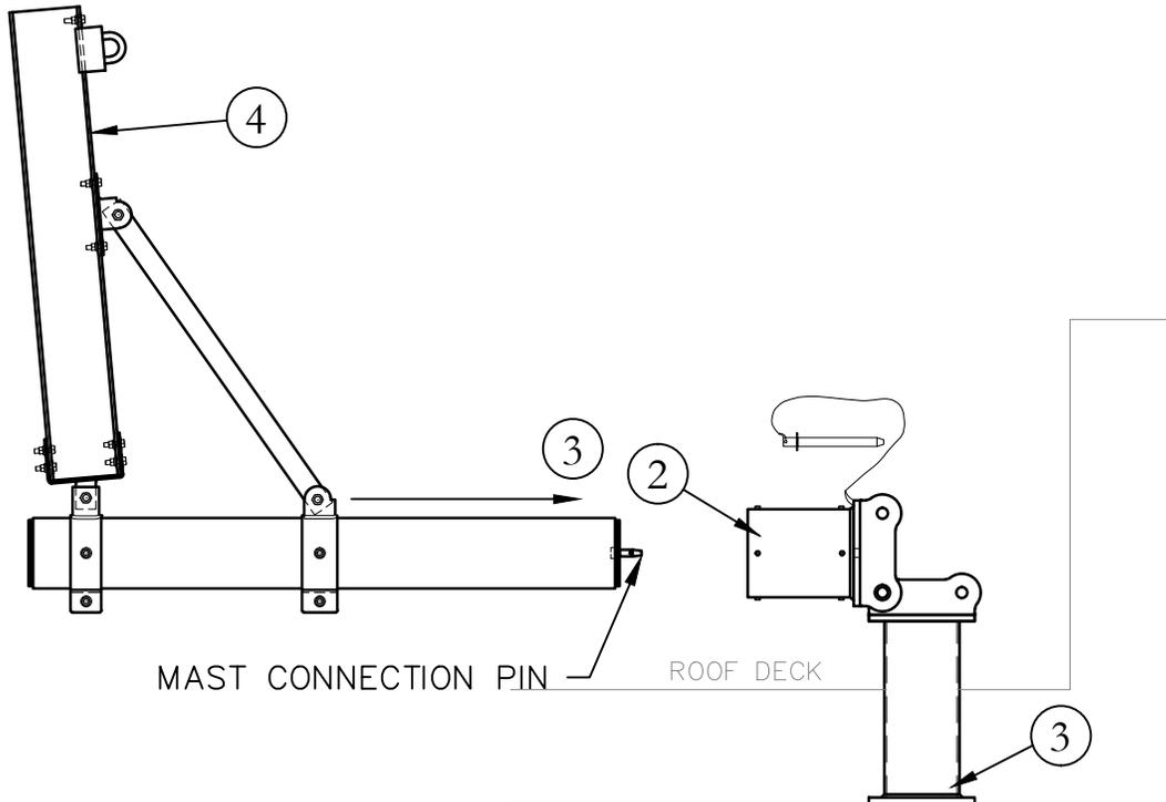
2. MOVE DAVIT ARM ASSEMBLY (#1) INTO THE SOCKET ASSEMBLY (#2) AS SHOWN. ONCE DAVIT ARM ASSEMBLY (#1) IS INSERTED INTO THE SOCKET ASSEMBLY (#2), INSTALL MAST CONNECTION PIN. MAKE SURE THE MAST CONNECTION PIN SAFETY CLIP IS INSTALLED AND IS FULLY ENGAGED.
